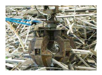
3 different tine shapes available: open, semi-closed (standard), closed.
